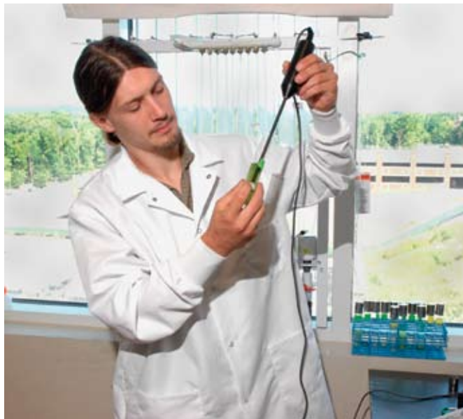
Chantry Johnson, a Mechanical Engineering senior, works with a light intensity probe that is used for gathering data from algae samples taken from a laboratory bioreactor.
