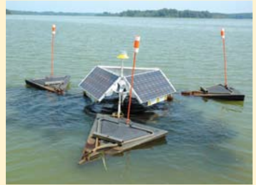
One of six solar bees that recirculate water in an effort to improve reservoir quality.
