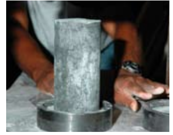
A 3"x6" cylinder of fly ash concrete in a universal testing machine.
