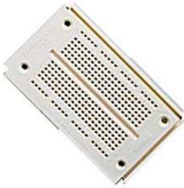
Figure 2. A small solderless breadboard. The row of holes on the outside edge is one node usually used to connect the power supplies. IC's are places across the groove in the center allowing 4 other connections to a single pin.
