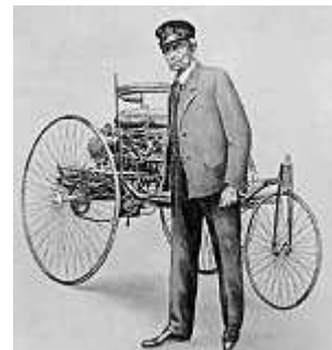
Karl Benz with the world's first automobile powered by an internal combustion engine.
